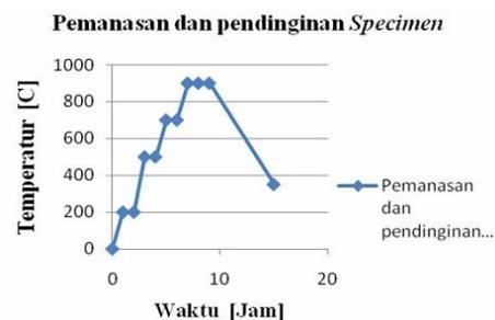
Gambar 1. Proses *pack carburizing*
